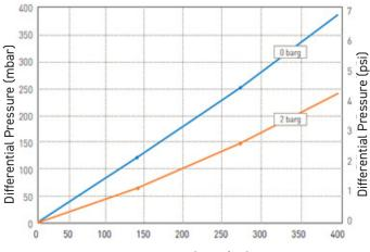
Flow per 10" cartridge (Nm $^{3}$  / hr) air @21 $^{\circ}$ C For A size filter, multiply dP by factor of 3 at same flow
